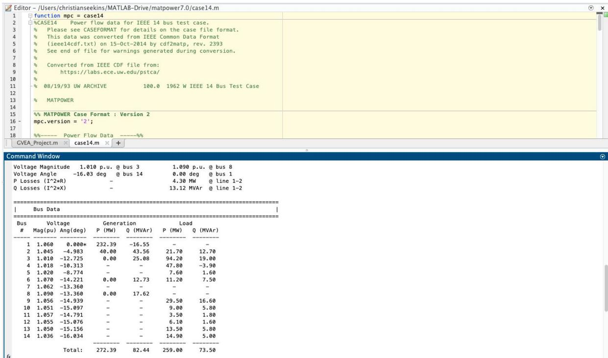
Figure 2: Matpower powerflow result example, case 14
