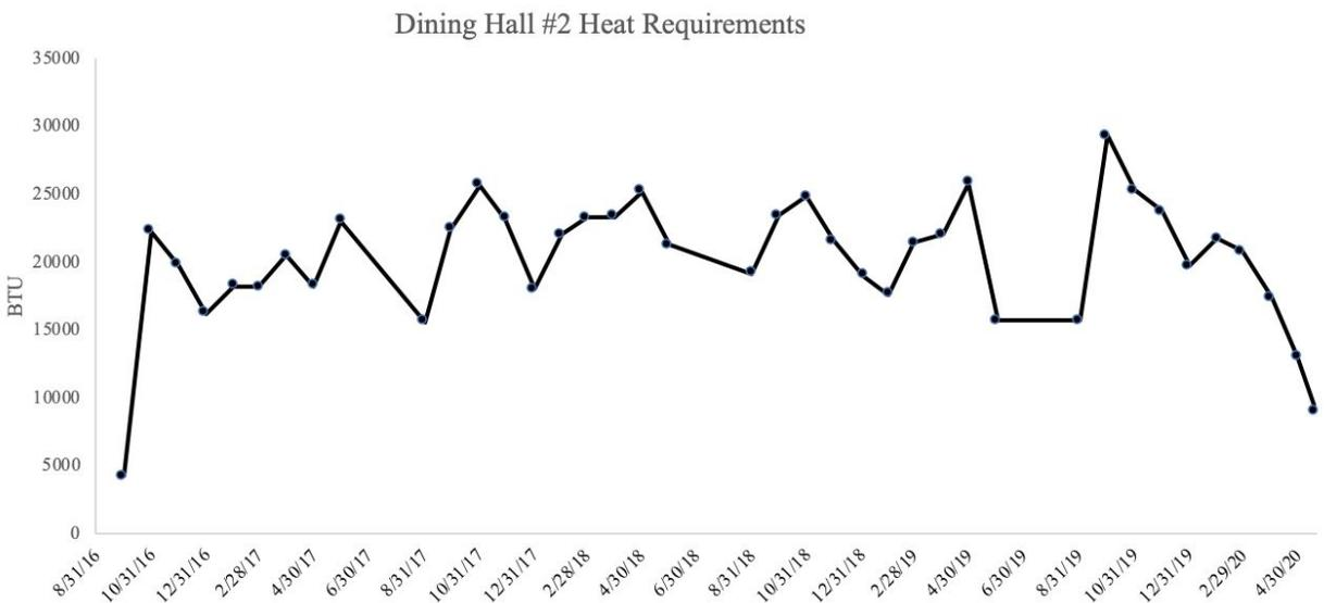
Figure 6. Heat data of Dining Hall #2 within the GILA campus. Compared to Figure 5, the heat profile does not vary significantly with season, indicating poor insulation and low energy efficiency.
