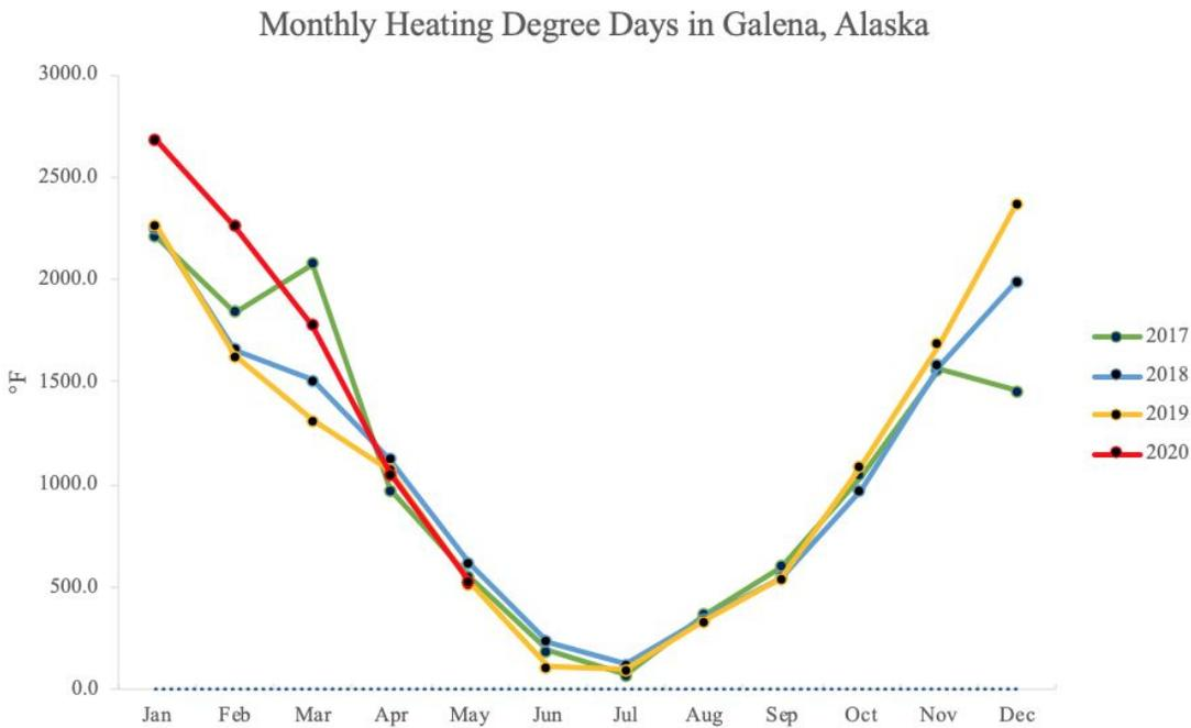
Figure 4. Total monthly heating degree days in Galena, formulated based on a 65 °F baseline.
