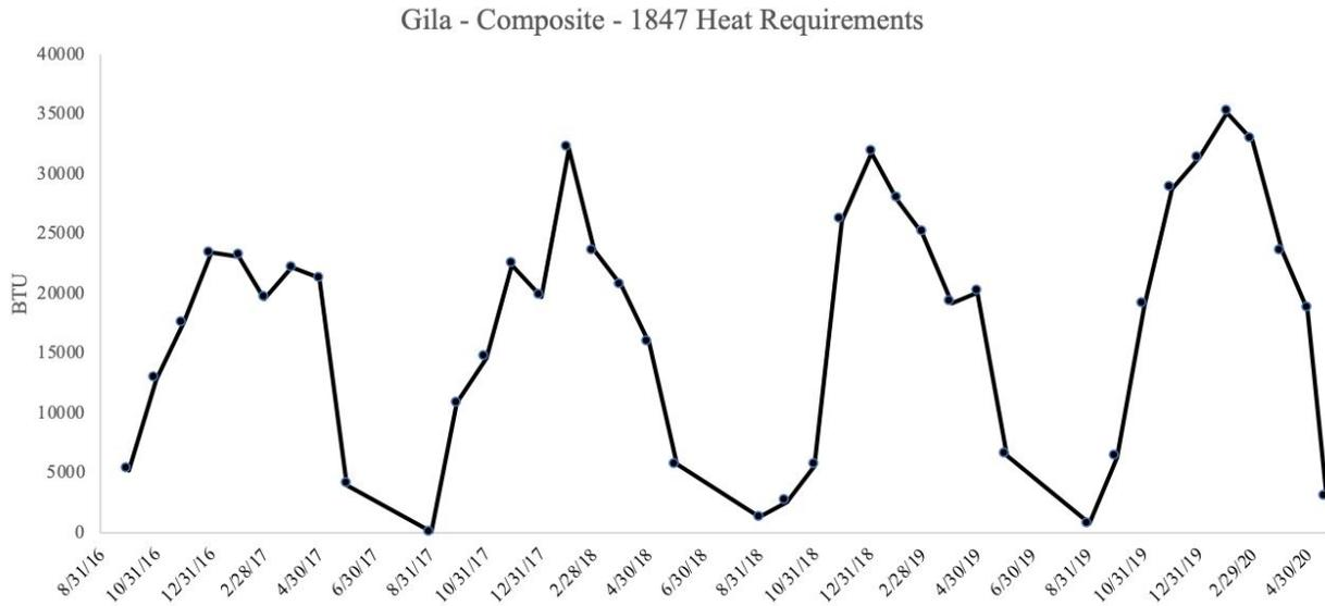
Figure 5. Heat data of the Composite building within the GILA campus. BTU readings span 2016-2020 and show a predictable seasonal heating profile.
